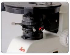
2. Rotate the polarizer to the zero position.
